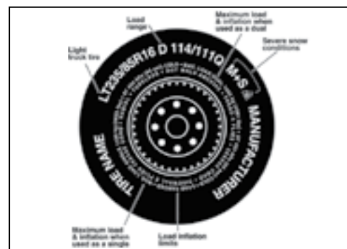
Figure 4: Typical Light Truck Tire Markings
